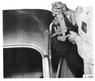
FITTING AND WELDING OF ROOF SHEET
