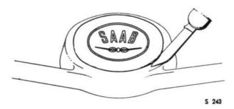
REMOVAL OF HORN BUTTON UP TO AND INCL. MODEL 1967
