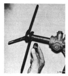
REMOVAL OF OUTER BALL SEAT FROM THE NUT, WHEN RE-SHIMMING.
