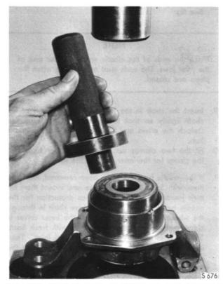
PRESSING IN THE BALL BEARING IN THE STEERING KNUCKLE, TOOLS 784030 AND 784075. THE MARK ON THE BALL BEARING FACING OUTWARDS
