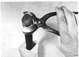
PLACING OF LOCK RING IN TOOL 784161
