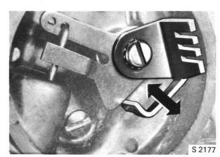
ADJUSTMENT OF THERMOSTATIC SPRING **LEVER TONGUE**
