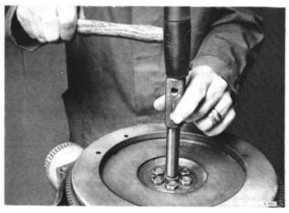
REPLACEMENT OF DISC-SHAFT BUSHING
