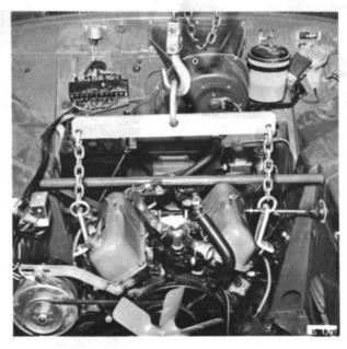
REMOVAL AND INSTALLATION OF ENGINE WITH LIFTING HOOK 786202
