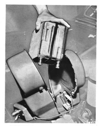
REMOVAL OF HEAT EXCHANGER
