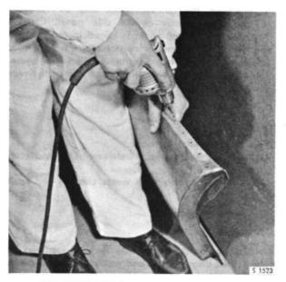
DRILLING HOLES FOR PLUG WELDING
