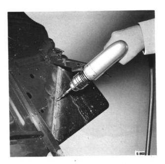
REMOVING SPOT-WELDS BY DRILLING
