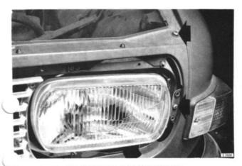
REMOVAL OF SCREWS, FRONT PANEL
