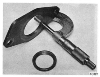
MEASUREMENT OF THRUST PLATE
