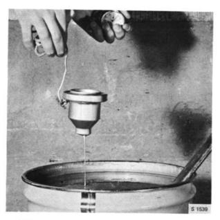
MEASURING VISCOSITY WITH AN SIS BEAKER
