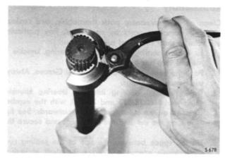
PLACING THE LOCK RING IN TOOL 784161
