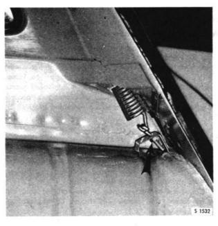
ADJUSTMENT NUT FOR TENSION OF TAILGATE BALANCE SPRINGS, SAAB 95
