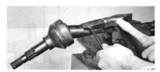
REMOVAL OF INNER DRIVE SHAFT FROM OUTER UNIVERSAL JOINT WITH TOOL 784202
