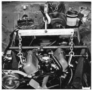
REMOVAL AND INSTALLATION OF POWER UNIT
