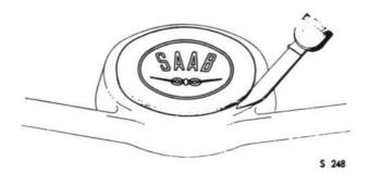
REMOVAL OF HORN BUTTON UP TO AND **INCLUDING THE 1967 MODEL**
