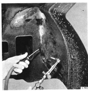
REMOVING UNDERSEAL COMPOSITION WITH A WELDING TORCH AND COMPRESSED AIR
