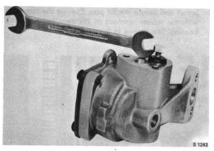
**REMOVAL OF RELIEF VALVE COVER PLATE**
